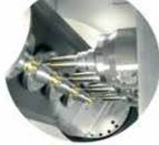
4 spindle, 4 axis: • SW BA400-4 (X:200mm - Y:500mm - Z:425mm)
